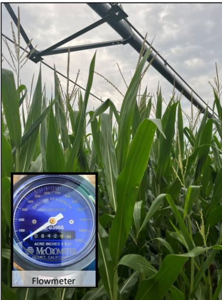
One of the requirements of drilling a new irrigation well (or any well that pumps over 50 gallons/minute) within the Nemaha NRD is that you must have a flowmeter. If you haven't heard of a flowmeter before, it is a tool that measures the rate at which water is being pumped and the cumulative volume of water that has been pumped.
